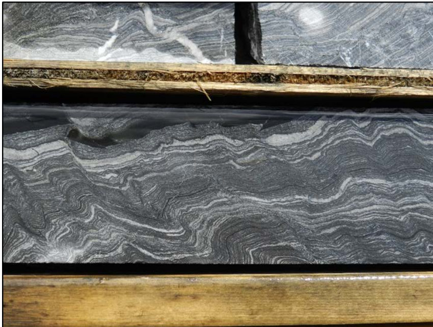
Figure 7-10: Minor Folds of Likely Tectonic Origin in Gray Facies Mineralization from Tom West
