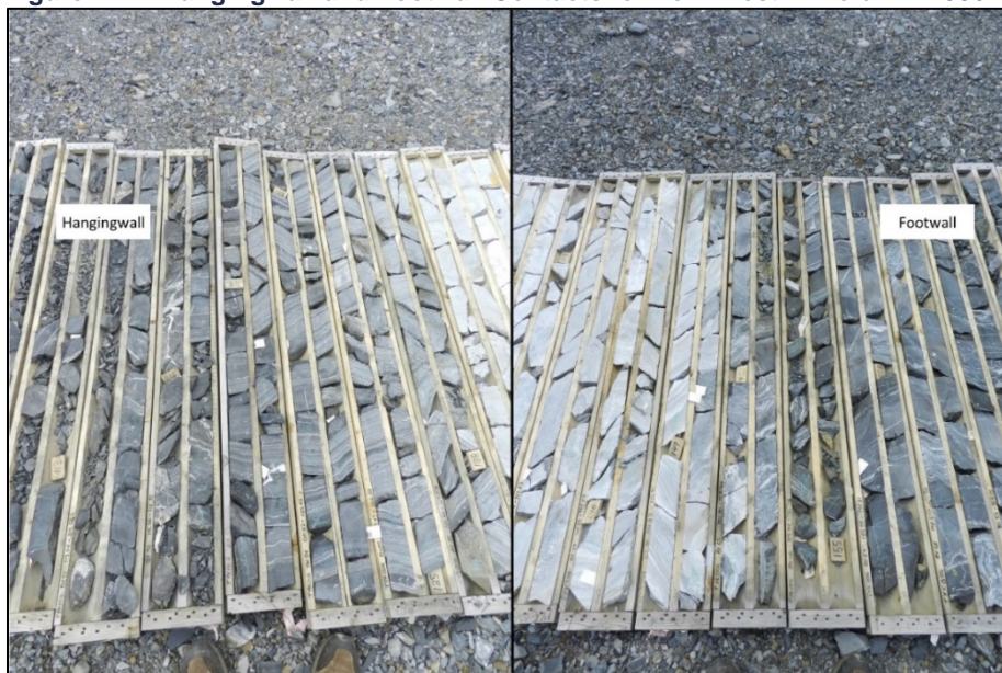
Figure 7-12: Hangingwall and Footwall Contacts for Tom West in Hole TYK-006 Drilled in 2011
